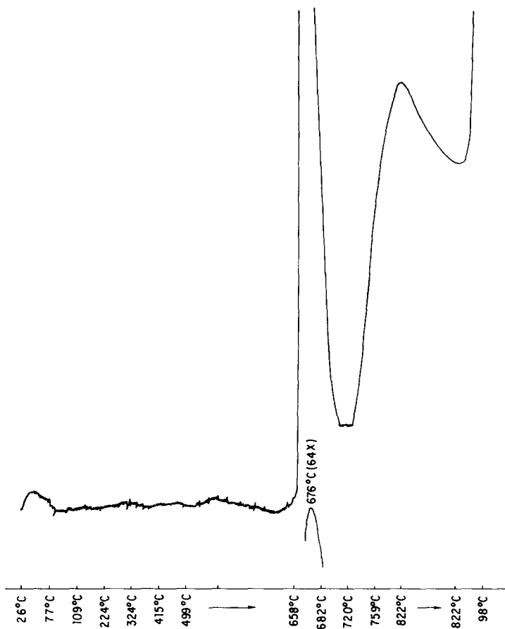
Fig. 2. Temperature-programmed reduction experiment for the Ni/Al 2 O 3 catalyst using 20% methane–nitrogen mixture at 10°C/min.
